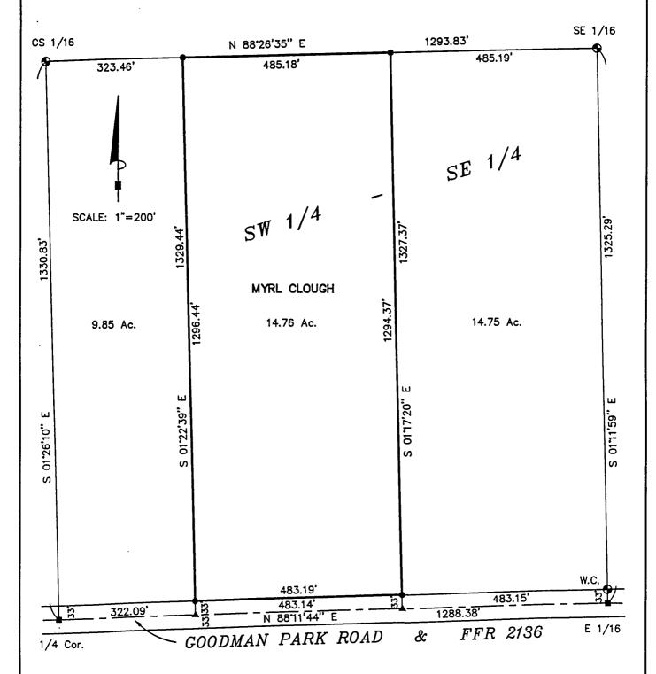
NOTE: BEARINGS ARE REFERENCED TO THE U.S.F.S. PLAT OF SURVEY OF SECTION 12, T35N, R15E
