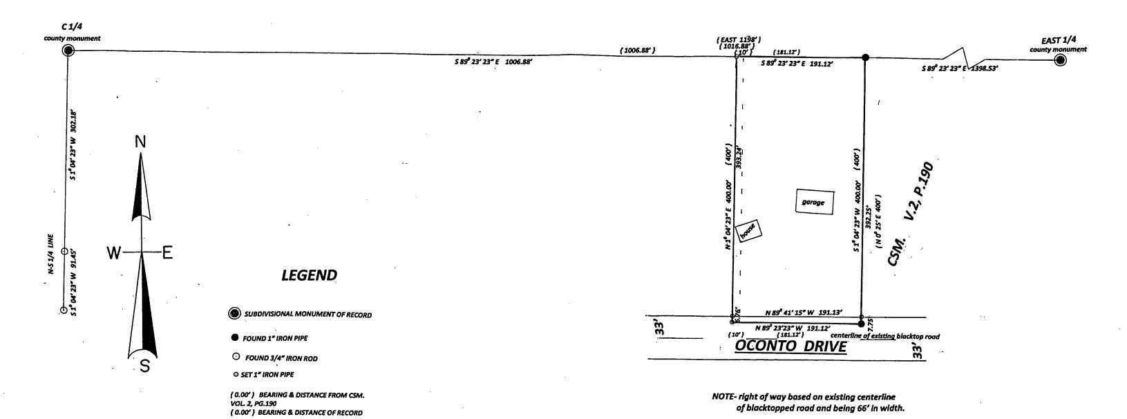
North is referenced to the E-W % line Being an assumed bearing of S 89° 23' 23" E.
