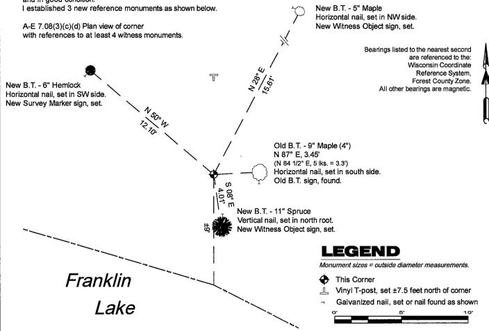
A-E 7.08(3)(e) 1859 Surveyor set a post, 1941 Surveyor set a 2" diameter iron post with a brass cap stamped to identify the corner location, subsequent Surveyors found similar. I found a 1.9" diameter galvanized iron pipe monument, with a 2.5" diameter brass cap stamped to identify the corner location in 2025.
