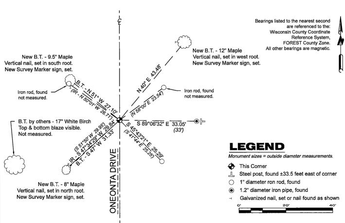
A-E 7.08(3)(e) 1857 Surveyor set a post, 2005 Surveyor found a 5/8" diameter iron rod, 2007 & 2011 Surveyor found a iron pipe. In 2024, I found a nail with a 0.4" diameter head.
