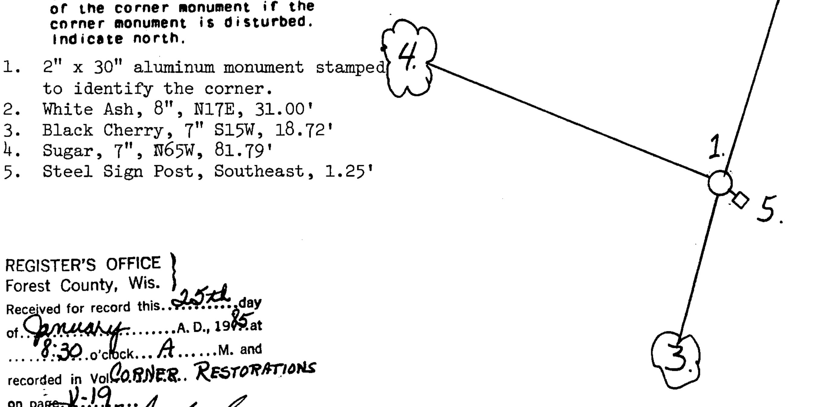
(e) Describe any material discrepancy between the location of the corner as restored or reestablished and the location of that corner as previously restored or reestablished by distance and direction. Show the discrepancy on the plan view drawing under (d), above. Show the distances between the corner as previously restored or reestablished and (1) the corner as restored or reestablished, and (2) to at least 2 of the witness monuments shown on the drawing in (d), above.
