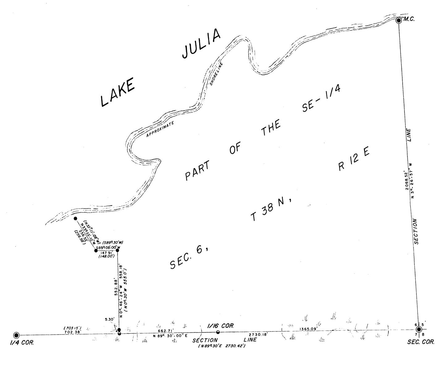
BEARINGS ARE BASED ON THE SOUTH LINE OF SECTION 6 WHICH BEARS N89º30'-00"E FROM PREVIOUS SURVEYS.
