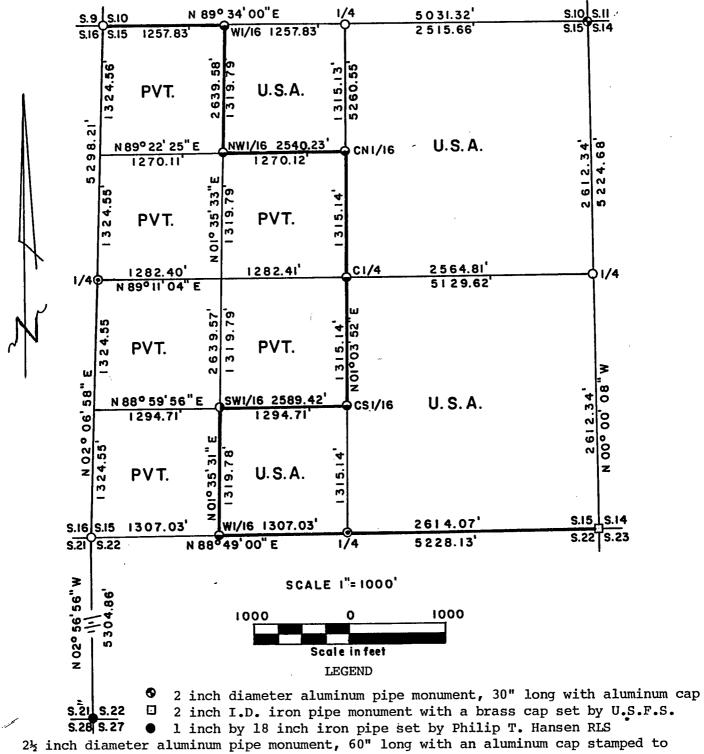
2½ inch diameter aluminum pipe monument, 60" long with an aluminum cap stamped to
