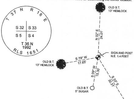
**BEARINGS MEASURED** WITHA HAND COMPASS
