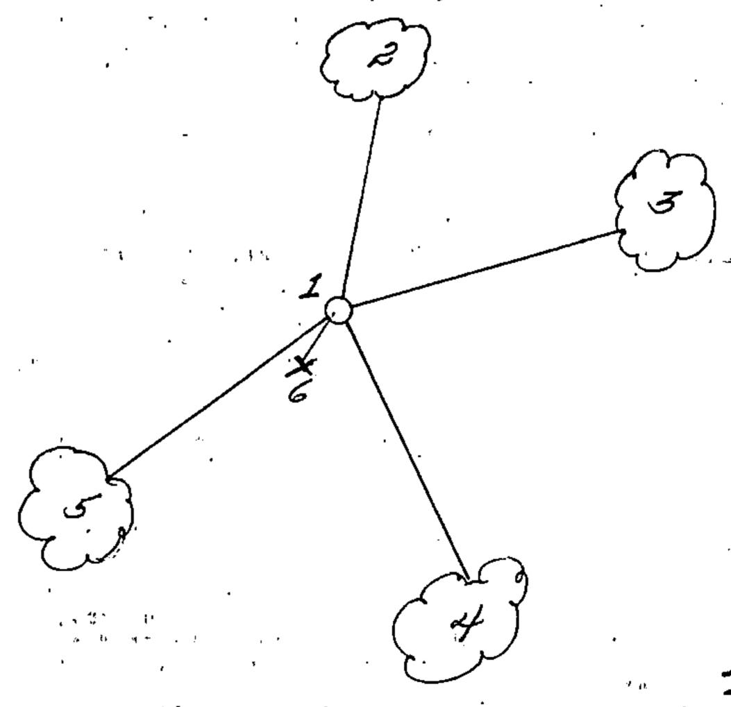
(a) Describe any material discrepancy between the location of the corner as restored or reestablished and the location of that corner as previously restored or reestablished by distance and direction. Show the discrepancy on the plan view drawing under (d), above. Show the distances between the corner as previously restored or reestablished and (1) the corner as restored or reestablished, and (2) to at least 2 of the witness monuments shown on the drawing in (d), above.
