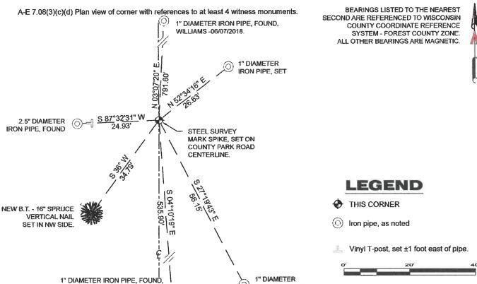
A-E 7.08(3)(e) 1865 Surveyor set a post, 2004 Surveyor set a PK nail, 2008 Surveyor found a PK nail, 2016 Surveyor found a Mag nail, 2018 Surveyor found a survey nail. I set a steel survey mark spike 3" long with a 1" diameter head at the location shown by the 2008, and 2018
