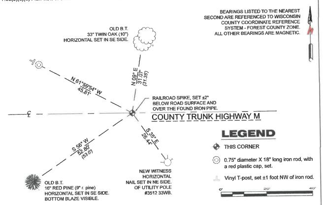
A-E 7.08(3)(e) 1865 Surveyor set a post, 1982 Surveyor found a 2" iron pipe, 2008 Surveyor found an iron pipe, 2023 surveyor found a 1" iron pipe. I found a 2" diameter iron pipe.
