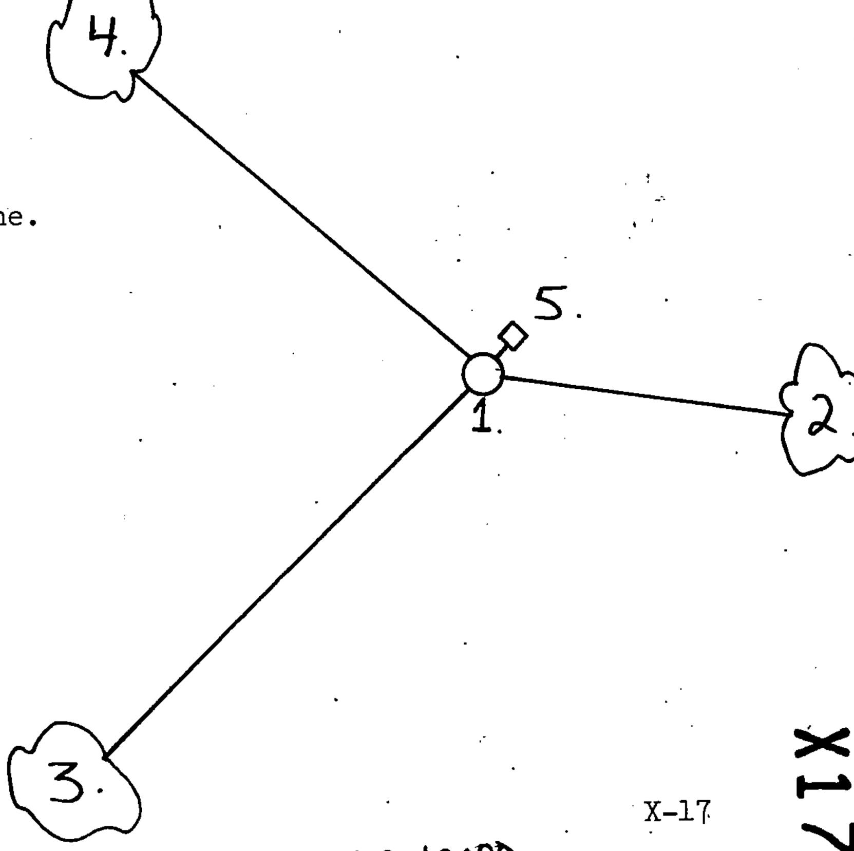
(e) Describe any material discrepancy between the location of the corner as restored or reestablished and the location of that corner as previously restored or reestablished by distance and direction. Show the discrepancy on the plan view drawing under (d), above. Show the distances between the corner as previously restored or reestablished and (1) the corner as restored or reestablished, and (2) to at least 2 of the witness monuments shown on the drawing in (d), above.
