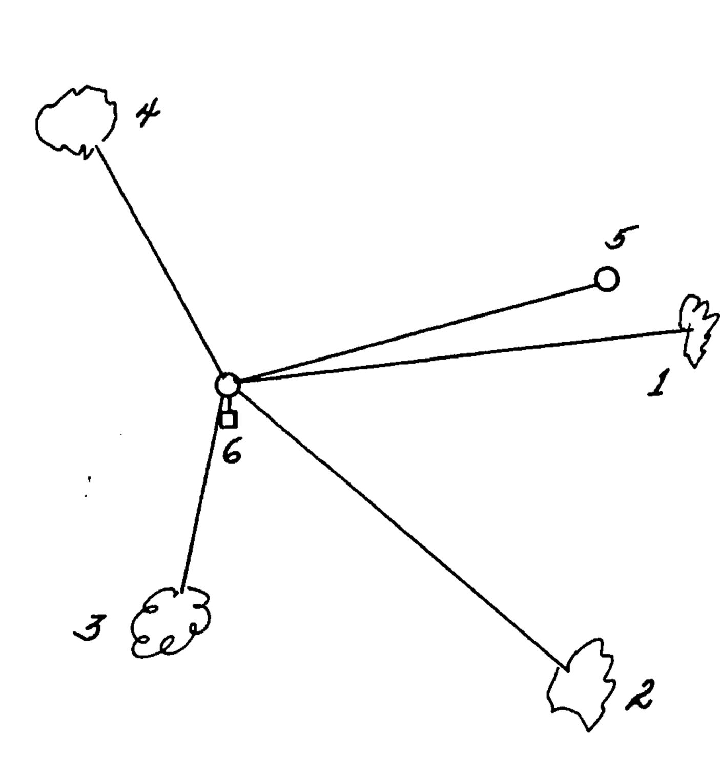
(e) Describe any material discrepancy between the location of the corner as restored or reastablished and the location of that corner as previously restored or reestablished by distance and direction. Show the discrepancy on the plan view drawing under (d), above. Show the distances between the corner as previously restored or reestablished and (1) the corner as restored or reestablished, and (2) to at least 2 of the witness monuments shown on the drawing in (d), above.
