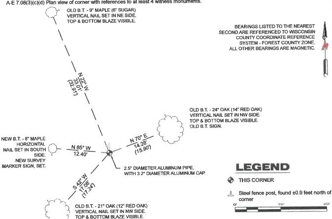
A-E 7.08(3)(e) 1859 Surveyor set a post, 1985 Surveyor set a 2 1/2" aluminum monument, 2005 & 2008 Surveyor found a 2" aluminum pipe monument. I found a 2.5" diameter aluminum pipe with a 3.2" diameter aluminum cap.
