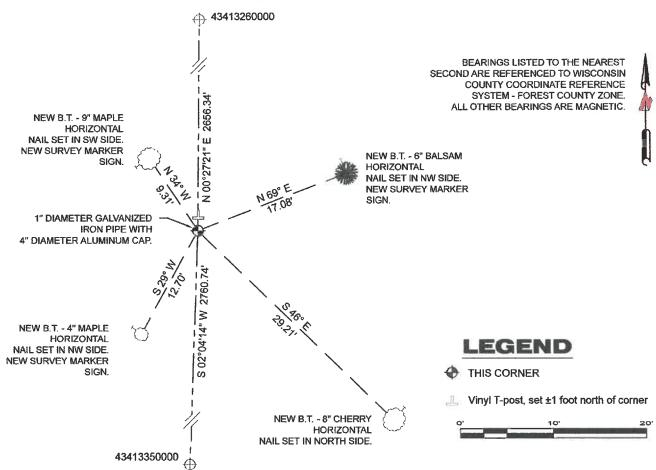
A-E 7.08(3)(e) 1865 Surveyor set a post, 1964 Surveyor set a galvanized iron pipe with an aluminum Kimberly Clark cap, 1993 Surveyor found a "county monument". 2023 - I found a 1" diameter galvanized iron pipe with a 4" diameter Kimberly Clark cap, stamped to identify the corner.
