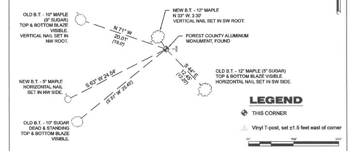
A-E 7.08(3)(e) 1865 Surveyor set a post, 1981 Surveyor set a 2.5" aluminum pipe with an alloy cap, subsequent surveyors found the same, as did I in 2023.
