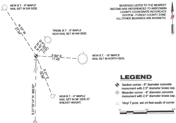
A-E 7.08(3)(e) 1857 Surveyor set a post, 2002 Surveyor found a 6" diameter concrete monument with a stamped brass cap. I found a 6" diameter concrete monument with a 2.5" diameter brass cap stamped to identify corner.
